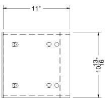
**CUSTOM TRUSS BRACKET** 1/2" ALUM PLATE (TYP) **BOLT HOLES MUST BE VERIFIED** TO FIT ACTUAL PURCHASED TRUSS ALL SEAMS FULLY WELDED
