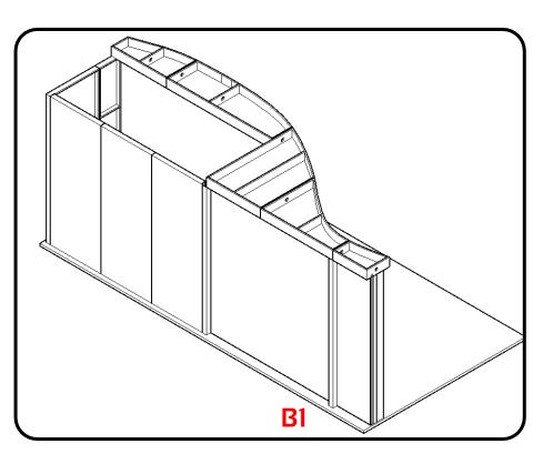
Once the Support pillar is in place, connect the Pillar topper to the pillar and canopy via drywall screw
