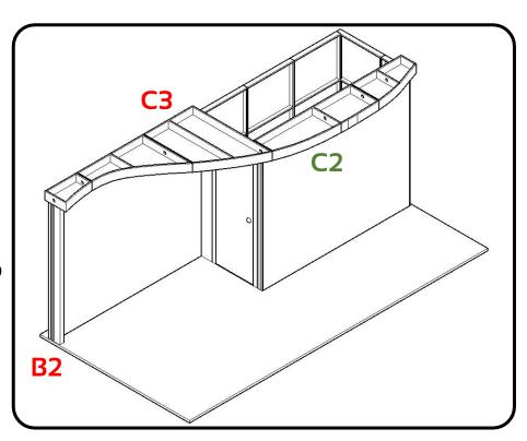
Bolt the SEG Frame into the canopy along the left, middle and right along the top of the frame
