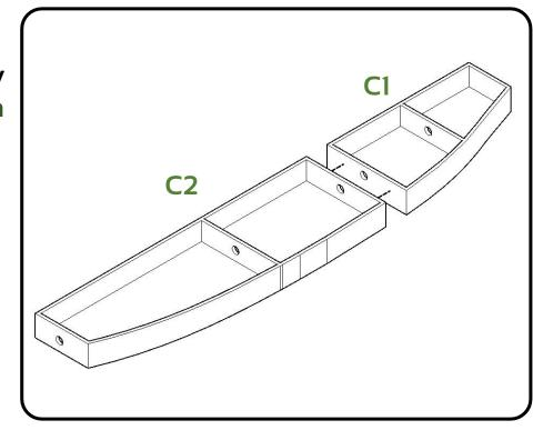
Carefully lift the canopy structure up and bolt into the closet structure. The bolt locations are located on the left and right sides of the closet canopy
